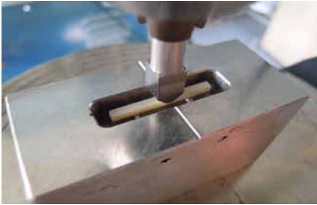
Fig 2 Bar-shaped specimen placed in a device designed for performing three-point bending test in accordance with ISO standard 4049/2000. The specimen was loaded at its center with a cylindrical-ended striker by the universal testing machine.
