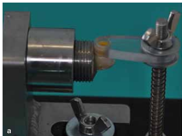
Fig 1 a. Specimen preparation for shear bond strength testing – specimen bonding on the target surface within a rubber mold. b. Schematic drawing of the specimen preparation.
